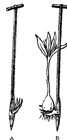
TOOL FOR EXTRACTING BULBS OF MEADOW SAFFRON.
