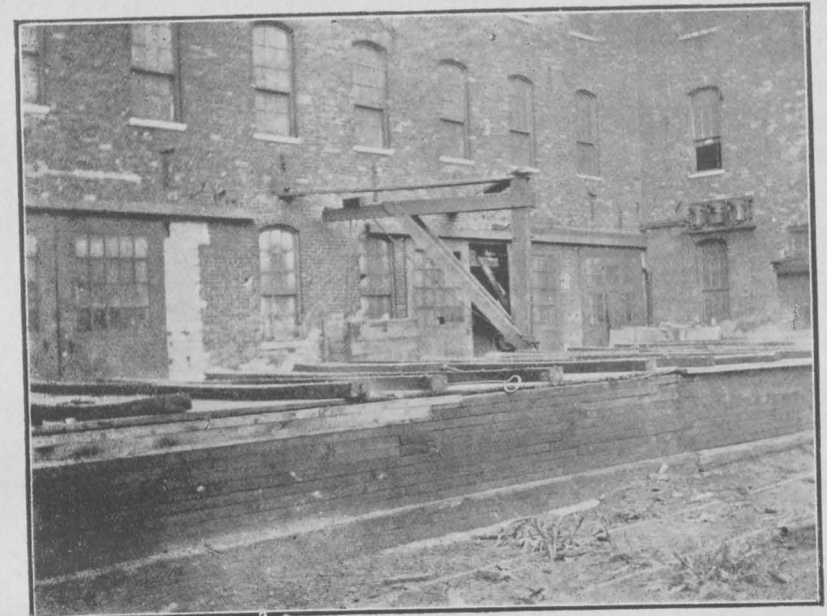
5. A BOILING TANK LINED WITH SHEET METAL AND PROTECTED BY A LUMBER OUTER WALL TO PREVENT RADIATION. THE COVERS ARE OF WOOD. NOTE THE SWINGING DERRICK FOR TRANSFERRING THE LOGS FROM THE TANK TO THE MILL.
