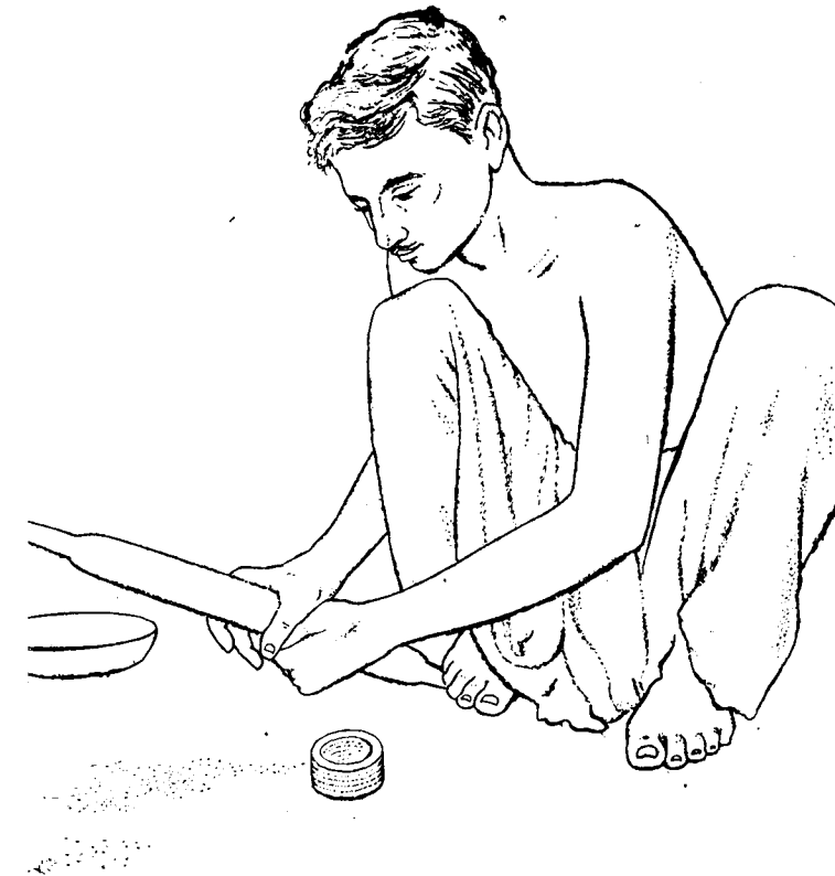
Polishing the inside of the bangles on a mandrel
