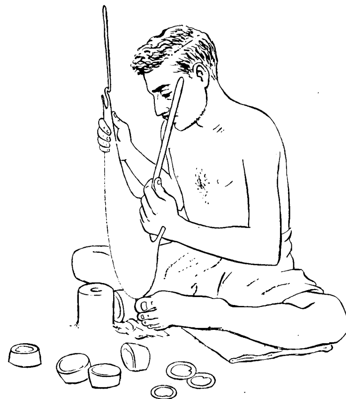
Cutting the upper part of the Conch shell into slices with a semi-circular saw
