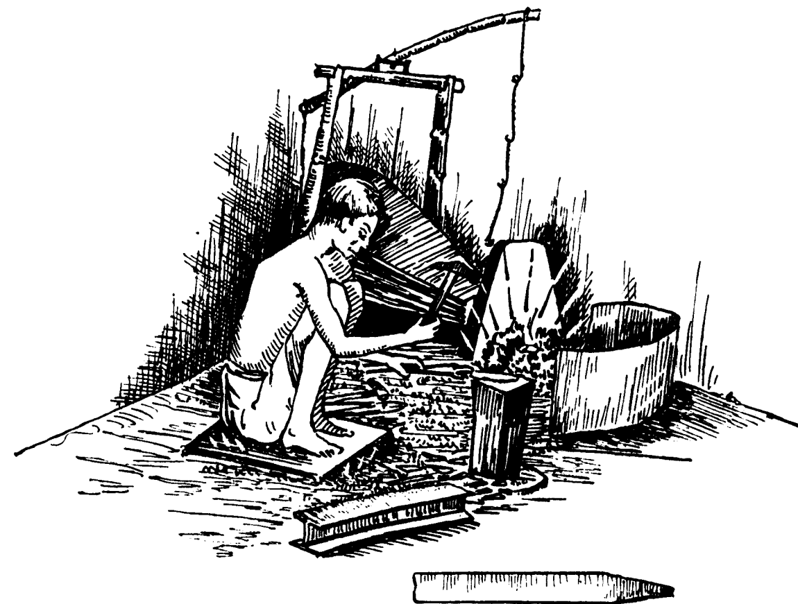
Sketch No. 72 Forging of blade (1)
