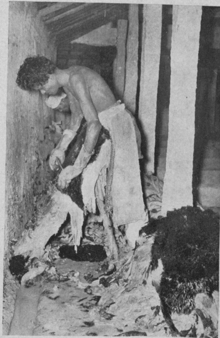
Placing the lime soaked skin on a vertical wooden plank, the worker wearing gloves to protect his hands from lime is busy removing the wool from the hide with a peculiar type of knife.
