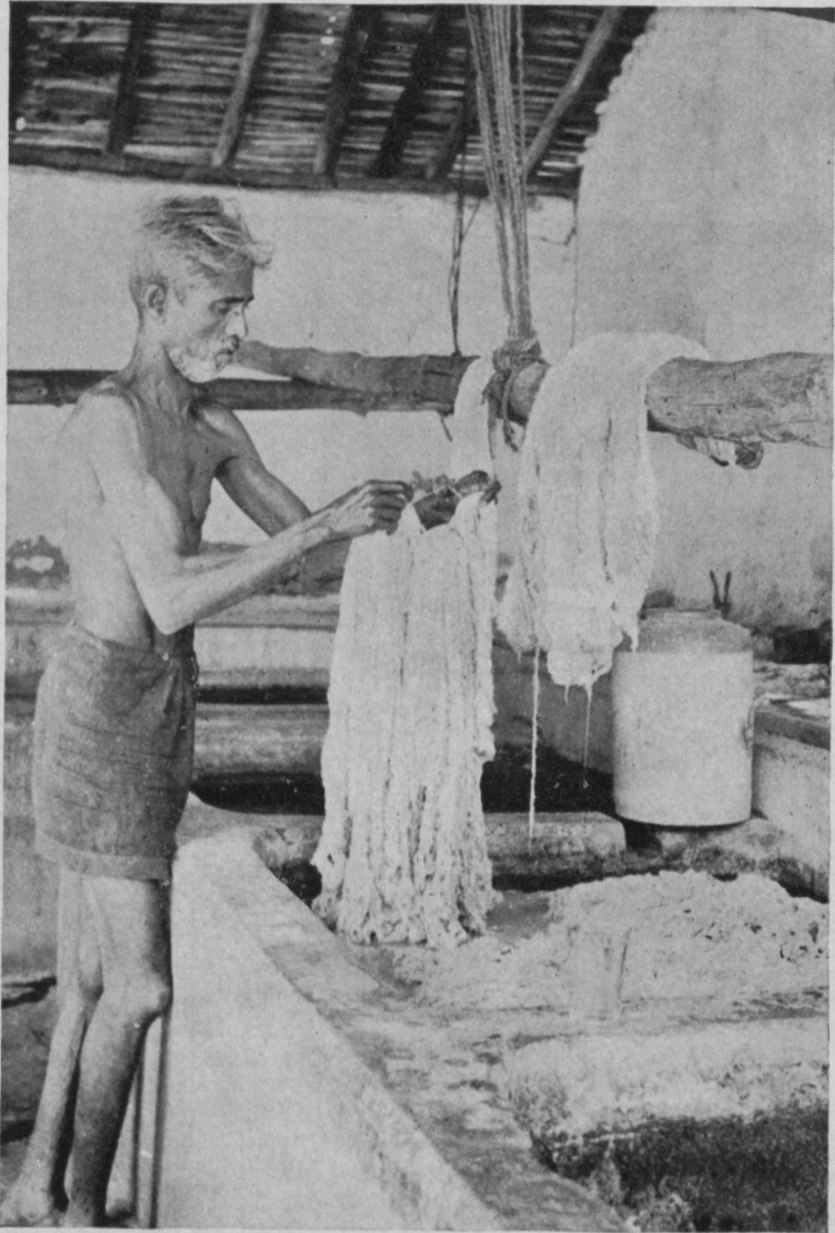
In the Drugget Factory at Walajapet, the dyer picks up the hanks from the tub, washed in the soap solution. (Note the China clay pot and glass used for mixing the chemicals)
