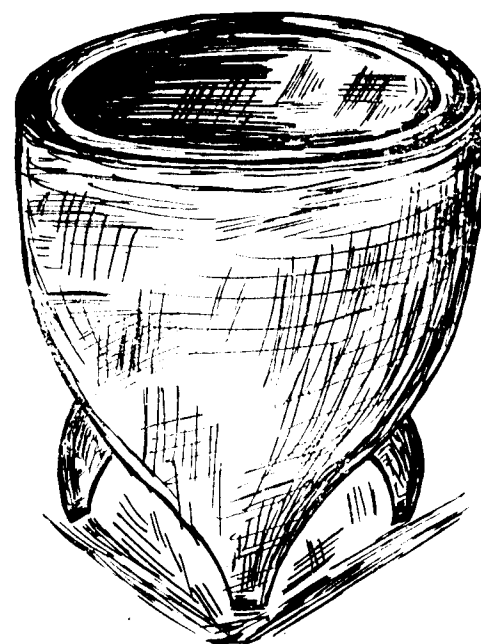
A U-shaped crucible ( gharia ) generally used in para casting method. It has three legs for being rested upon, so that it might not fall on one side.
