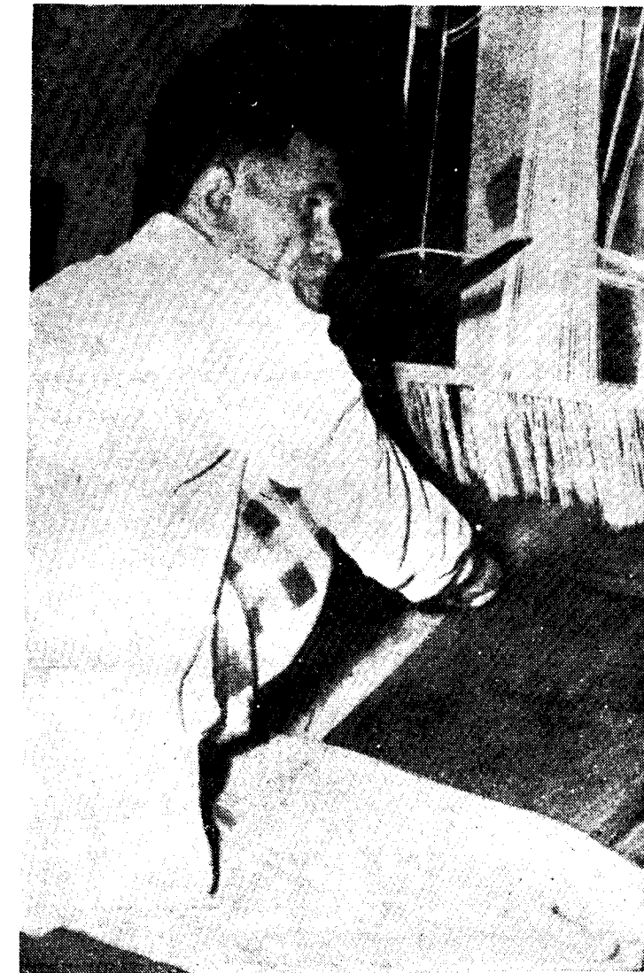
Plate 9. Warp twisting on loom.
