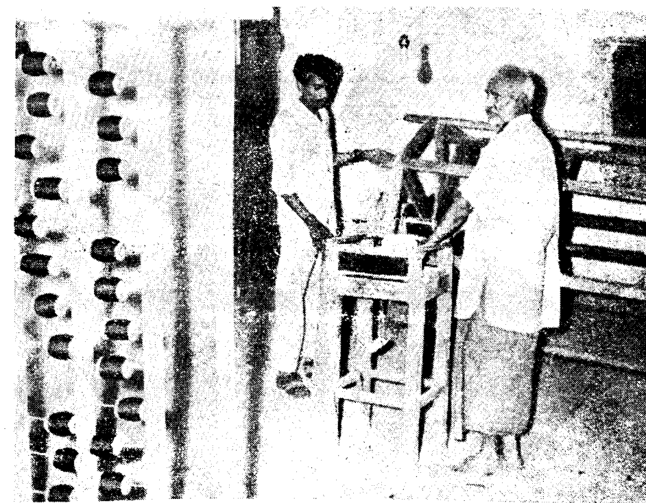
Plate 7. Warping in progress on drum-winding machine.
