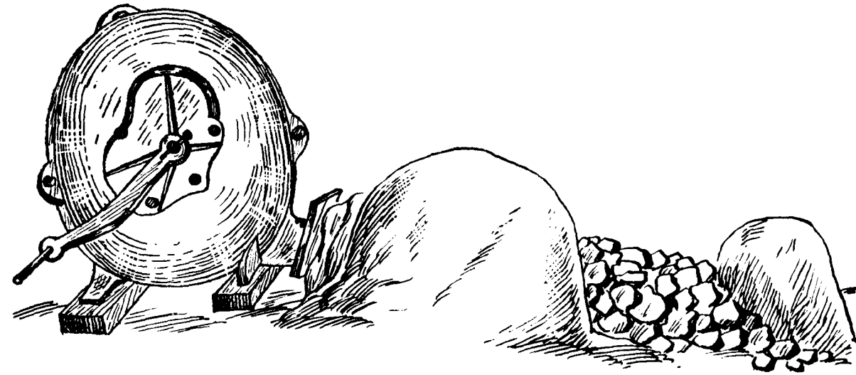
Rotary blower fitted to the forge
