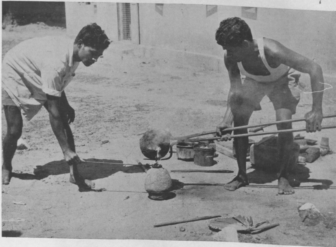
The crucible with the molten metal is lifted by the help of the tongs and poured into the hollow mould. Note the other moulder keeps over the mouth of the mould a dipped castor oil cloth rolled on an iron rod to keep the pouring molten metal temperature steady..
