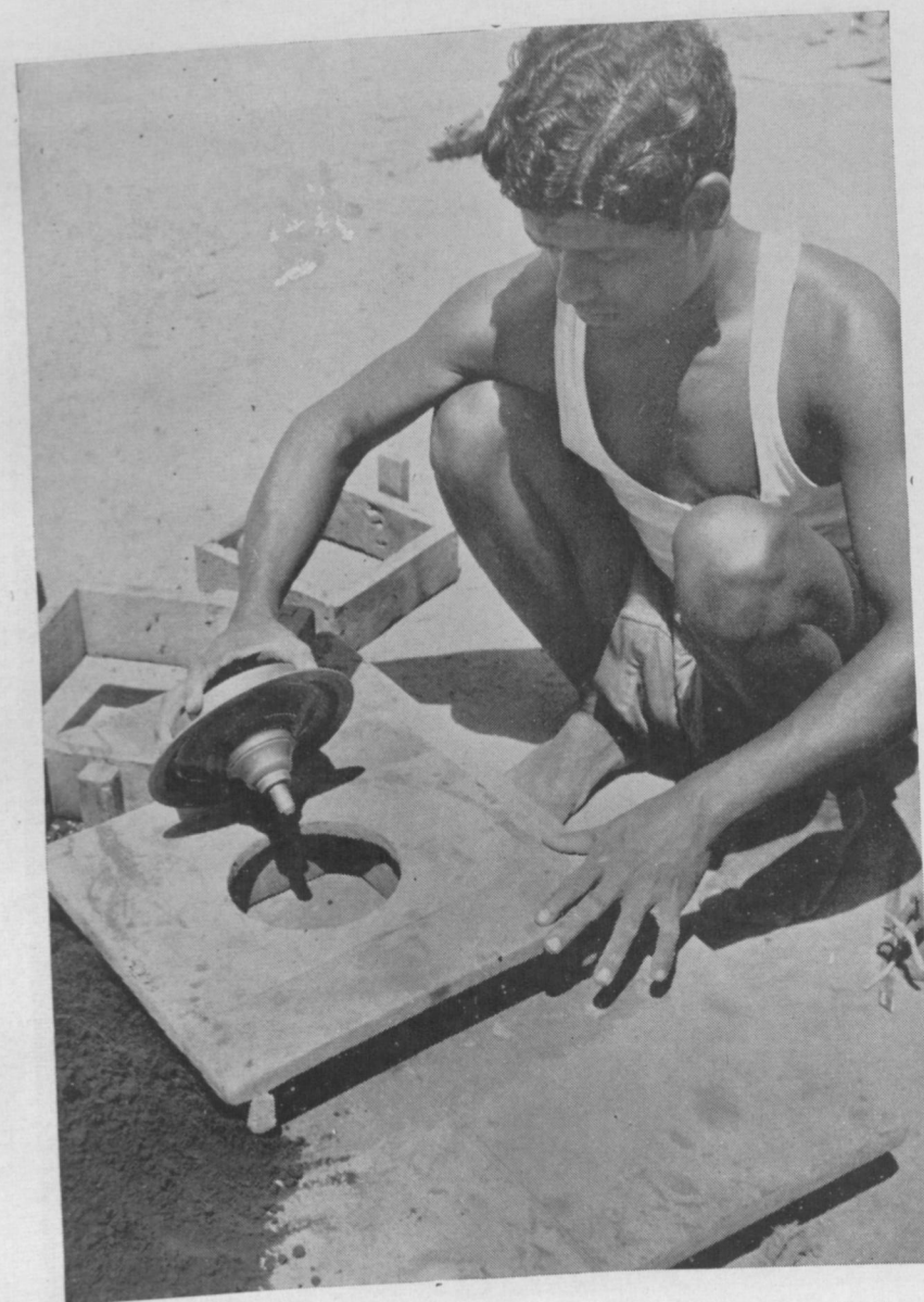
The pattern of the Kuthuvilakku base is being placed in centre upside down over a hole on a wooden plank.
