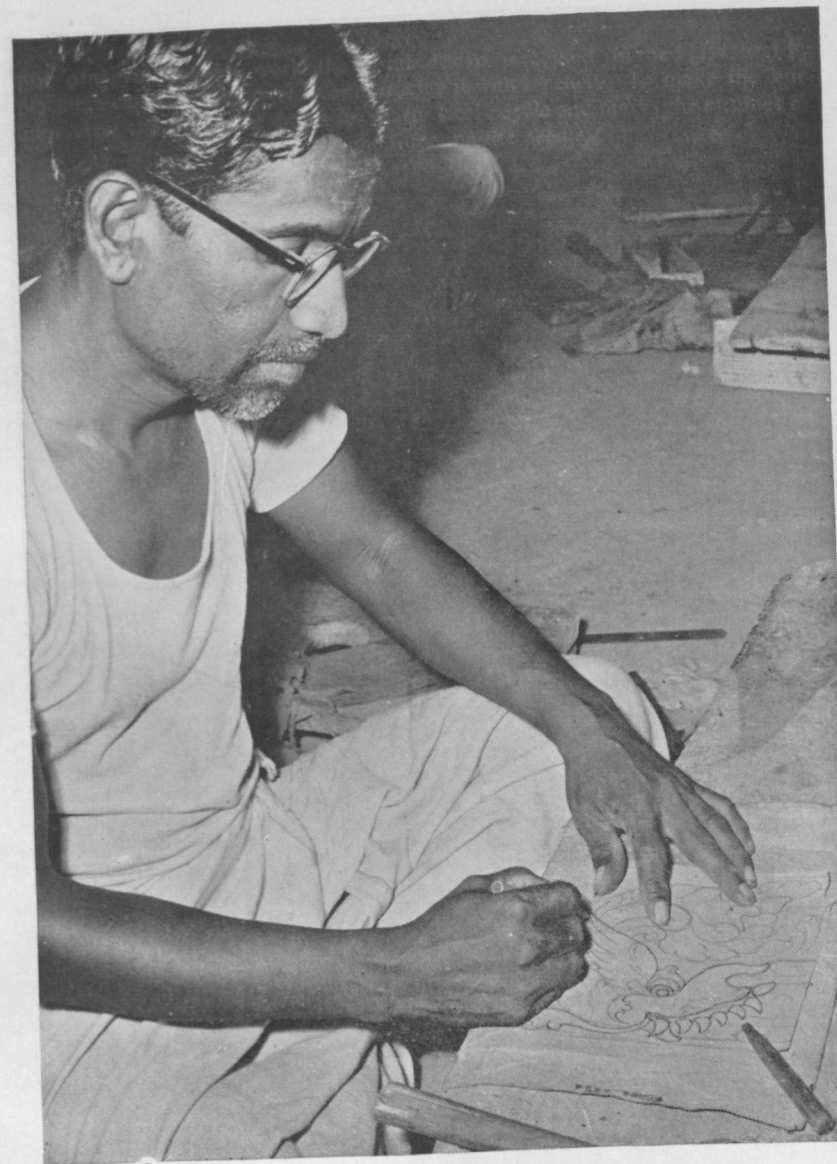
For ornamental sheet work the floral design is copied on the brass sheet by placing a carbon paper over it and tracing it with a pencil. To make the outlines clear the Sthapathi holds a sharp steel needle and marks the outlines by applying some force on the needle.
