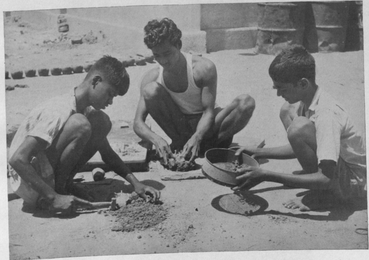
Some of the moulders are busy preparing the mud for loam moulding process at the left. The dried vandal sand is broken up with a hammer, in the centre, jute fibre is cut into small bits and at the right, the broken sand is sieved to remove its impurities.
