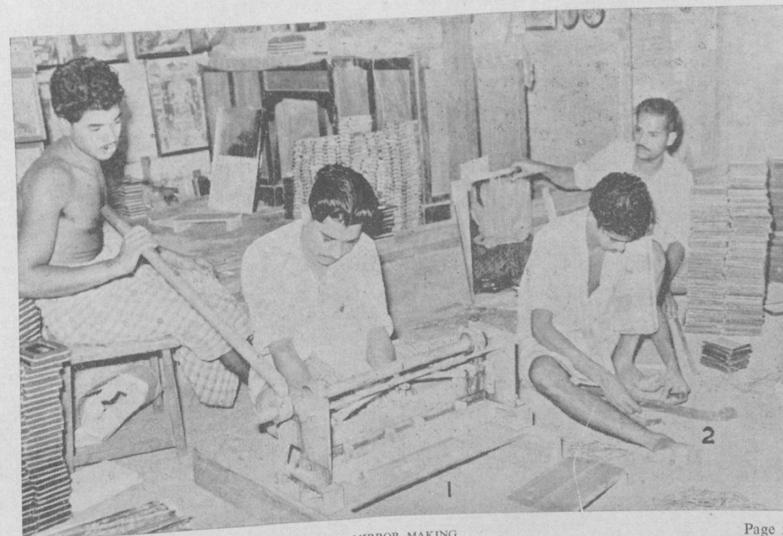
Pl. 34 MIRROR MAKING 1. MAKING DESIGNS ON THE TIN SHEETS FOR FIXING ON THE SIDES OF THE MIRROR 2. FIXING HOOKS ON ORDINARY MIRROR Page 53
