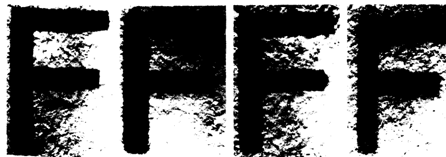
Fig. 3: Fixation of the stamping ink methylviolet on natural aged rag paper. a) Untreated. b) After immersion in water (20 min). c) After fixation by cyclododecane (solution in petroleum solvent 100/140, both sides) and immersion in water (20 min). d) After fixation by Me-sitol NBS 6% (brush, both sides) and immersion in water (20 min)
