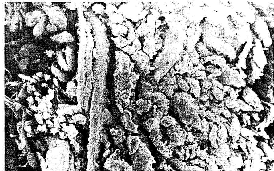
Fig. 7. Russian parchment, 13 th century (x200). Cross section disposed vertically. The absence of heterogeneous coating is evident.
