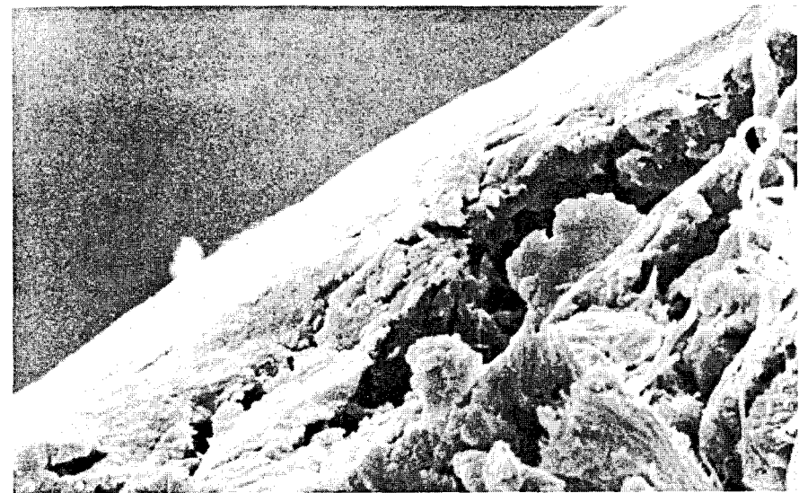
Fig. 6. Same as Fig., 5, enlargement 6000 fold. It can be seen that the coating on the hairside is analogous to that on the fleshside.
