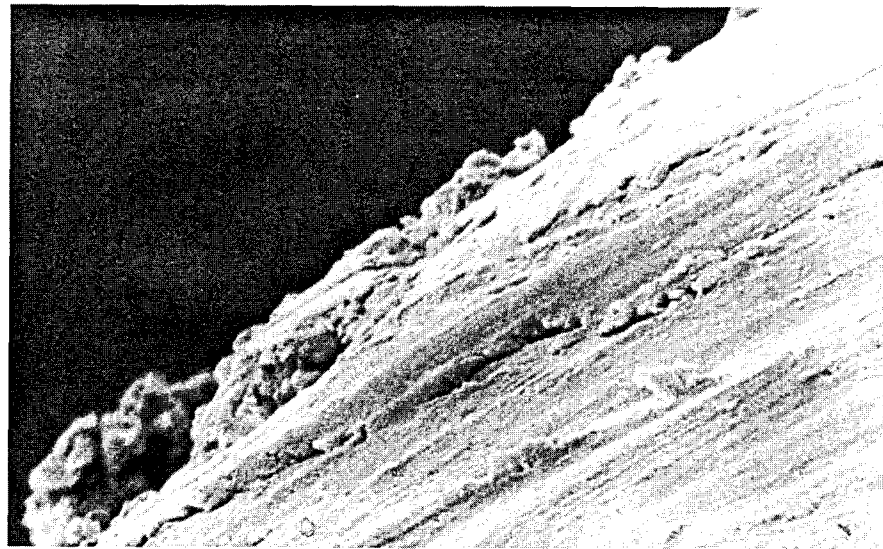
Fig. 4. Greek parchment, 14 th century (x6000). This high enlargement helps to see clearly the amorphous structure of the surface coating.
