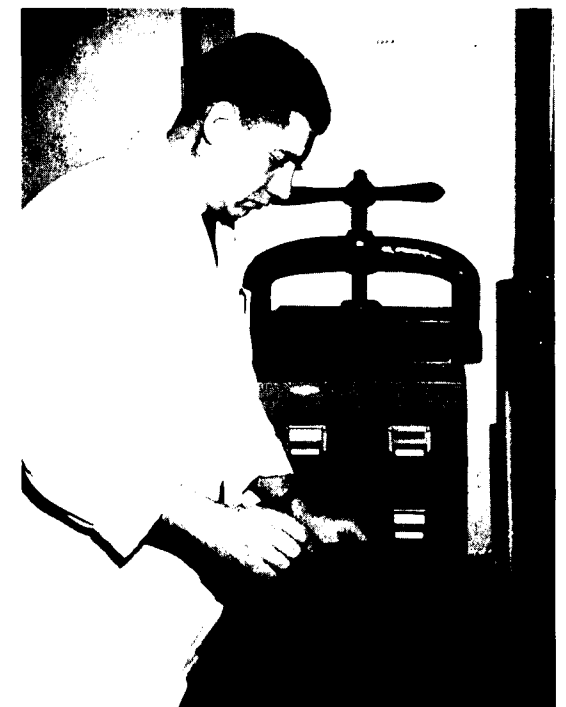
PLATE 8. Palm-leaf being put between release-coated paper before pressing.
